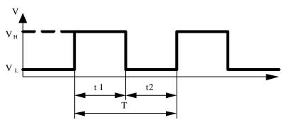
$$T = \frac{1}{f_{\text{PWM}}} = t1 + t2 \, (\text{sec}) \quad .$$
