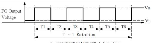
T= T1+T2+T3+T4+T5+T6=1 Rotation  $T = \frac{60}{rpm}$
