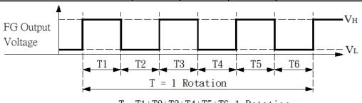
T= T1+T2+T3+T4+T5+T6=1 Rotation  $T = \frac{60}{rpm}$
