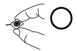
Don't pull fan with lead wires.
