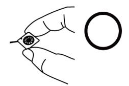
Don't pull fan with lead wires.
